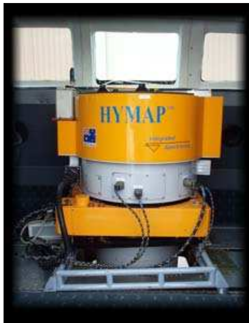
Figure 61: imageur hyperspectral HYMAP
