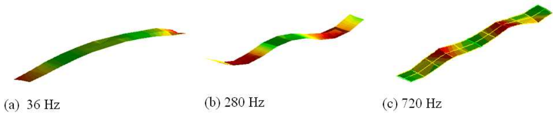
Figure 3.6 Mode shapes of composite beam calculated by the Polymax method (a) first bending, (b) second bending and (c) third bending
