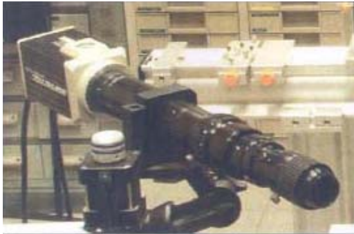
Figure 4.9: Shadowscopy: camera and extended objective
