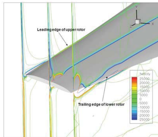
Figure 8.43: Axial vorticity at the upper blade tips
