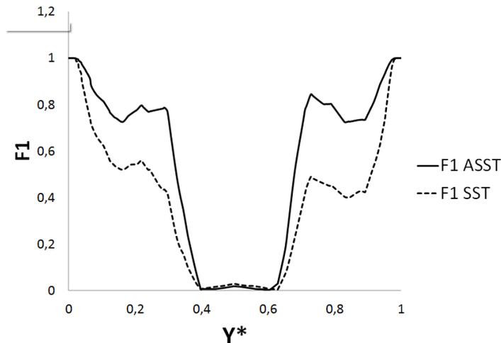
**Figure 5.9 - ASST vs SST model computed  $F_1$  function in the mixing zone central  $Y$  profile**
