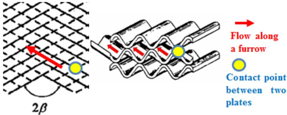
Figure 2.10 - Furrow and Contact Point visual definition
