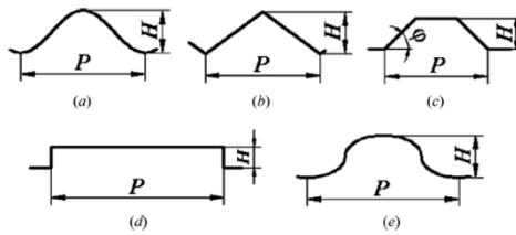
Figure 2.31 - Corrugation profiles<sup>61</sup>
