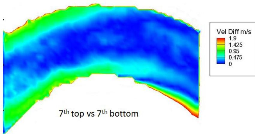
Figure 4.58 - PIV Flow symmetry evaluation: velocity field
