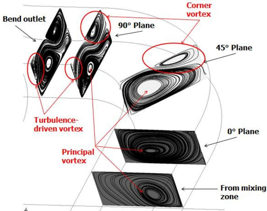
Figure 5.23 - In-bend flow ASST computed secondary motion evolution
