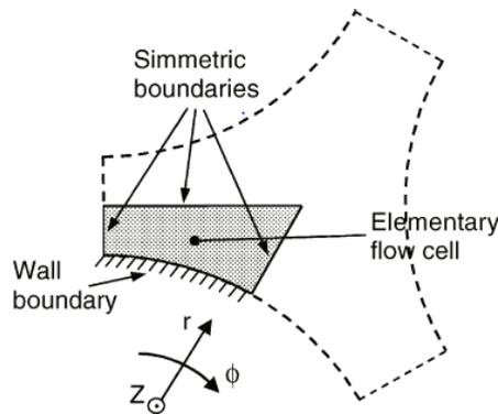
Figure 3.34 - Tight lattice rod bundle test configuration<sup>87</sup>
