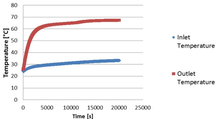
Figure 4.74 - "Low heat flux" case thermal transient evaluation
