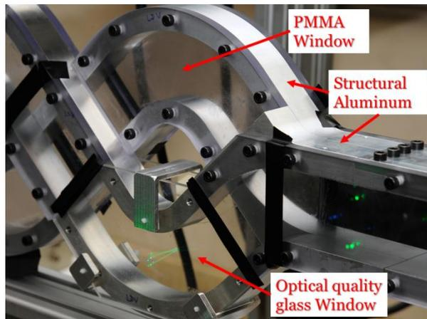
**Figure 4.4 - LDV test section material description**
