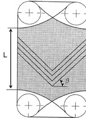
Figure 2.9 - Alternative geometrical definitions <sup>20</sup>
