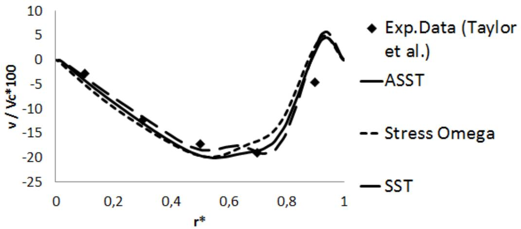
Figure 3.23 - AA line outlet section radial velocity distribution
