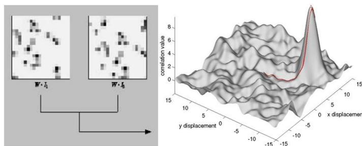
**Figure 4.39 - Example of PIV pixel cross-correlation**
