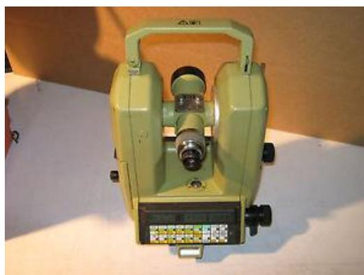
**Figure 4.15 - Theodolite used for laser calibration**
