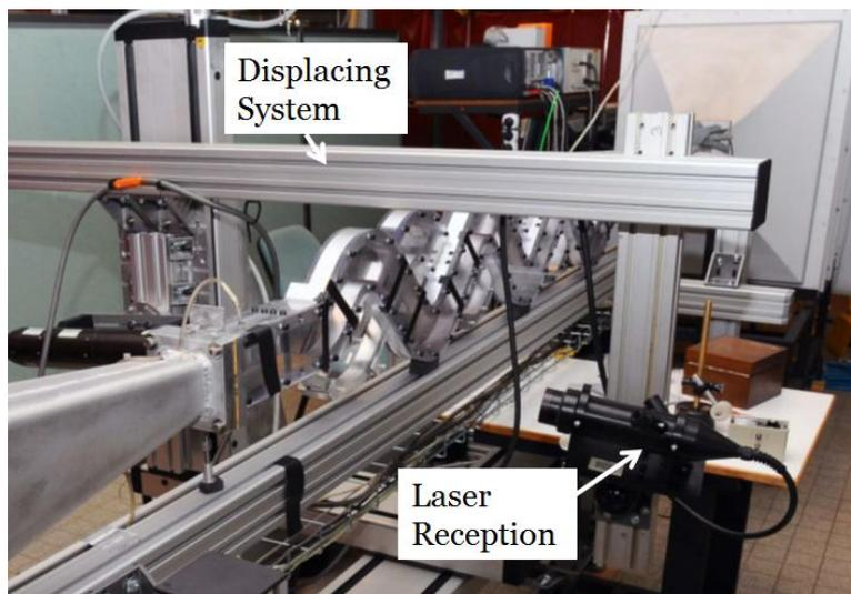
**Figure 4.8 - LDV displacing system and laser reception**
