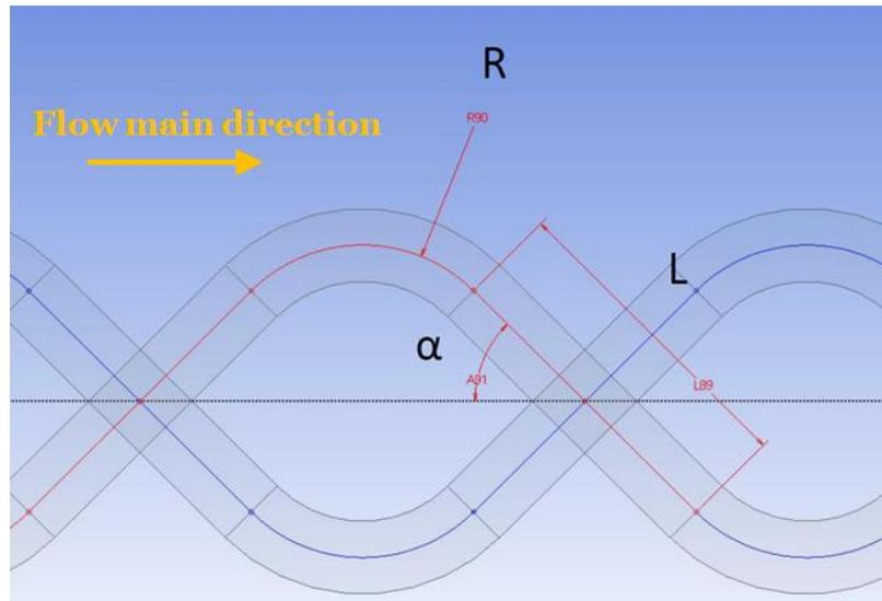
Figure 2.47 - Channel main geometrical parameters
