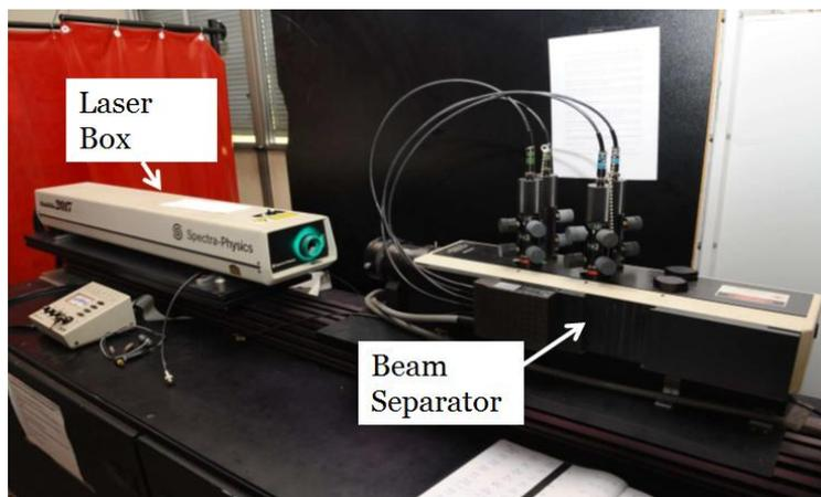
**Figure 4.6 - LDV Laser generator**
