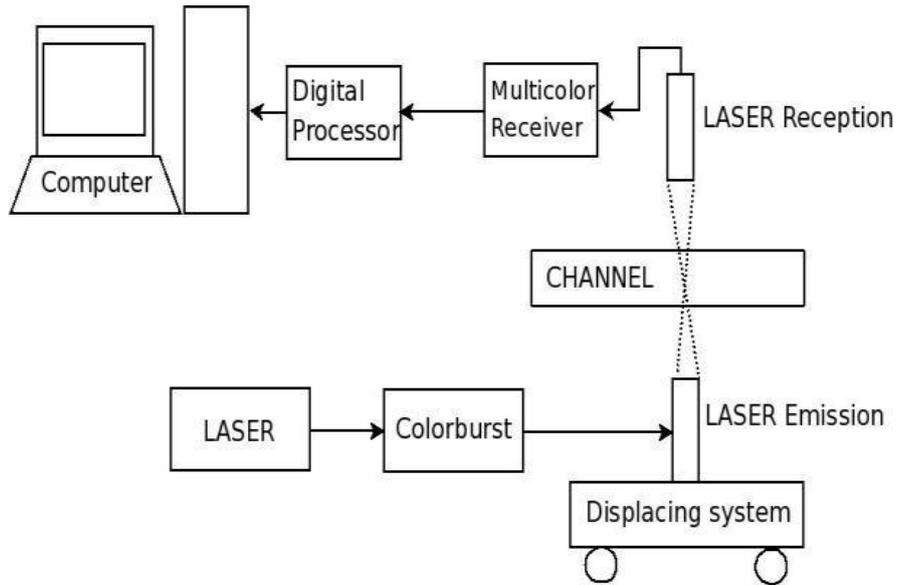
**Figure 4.5 -General scheme of the LDV experimental facility**
