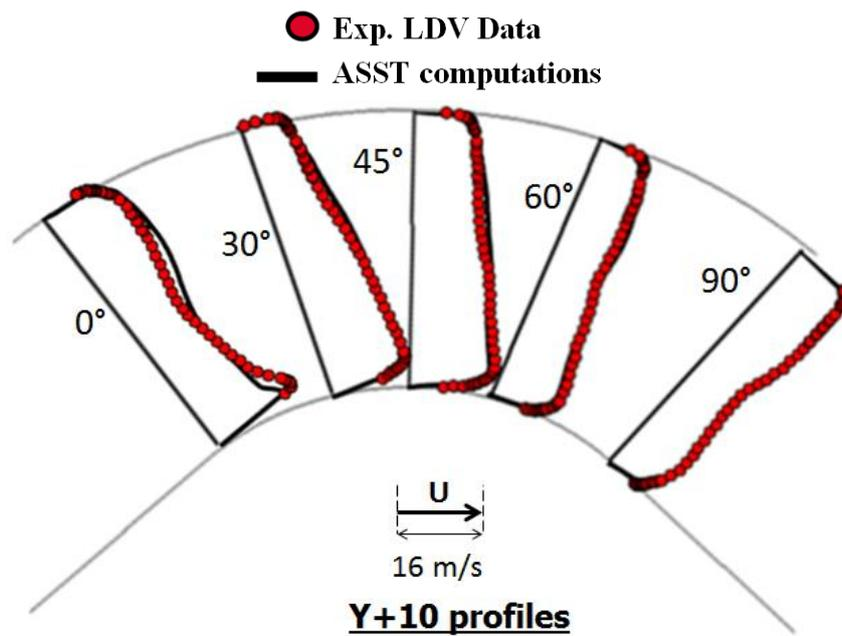
Figure 5.11 - LDV/ASST Y+10 principal velocity profiles for in-bend flow
