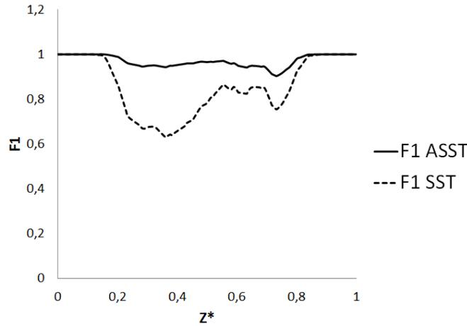
**Figure 5.8 - ASST vs SST model computed  $F_1$  function in the in-bend  $45^\circ$   $Y_0$  profile**
