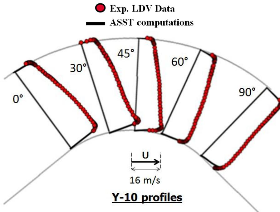
Figure 5.12 - LDV/ASST Y-10 principal velocity profiles for in-bend flow
