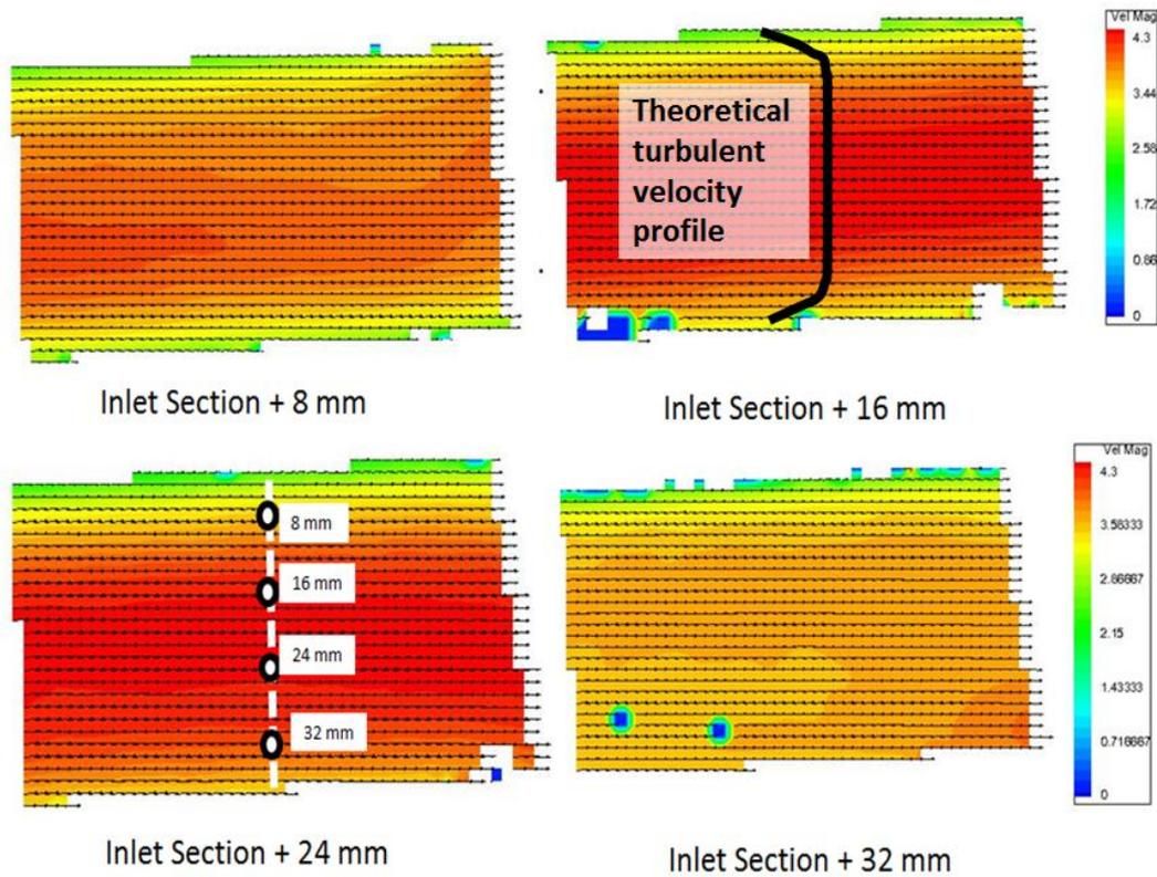
**Figure 4.54 - Inlet Flow Velocity field distribution**
