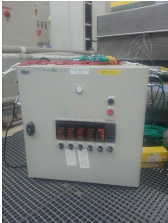
**Figure 4.66 - VHEGAS heating plates control system**
