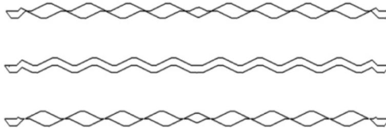
**Figure 2.8 - Hydraulic channel cross-section at different axial locations**<sup>19</sup>
