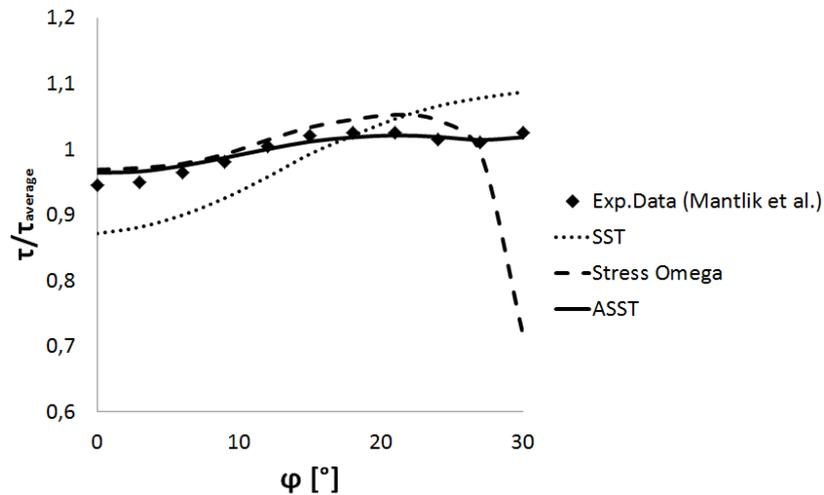
Figure 3.36 - Non-dimensional wall shear stress versus angular position
