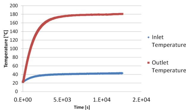
Figure 4.71 - "High heat flux" case thermal transient evaluation
