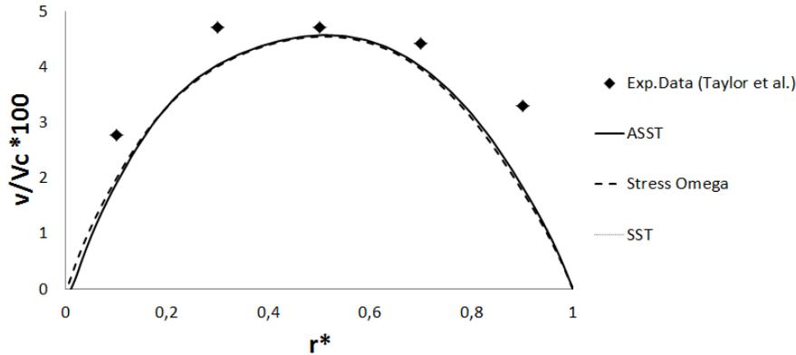
**Figure 3.20 - AA line inlet section radial velocity distribution**
