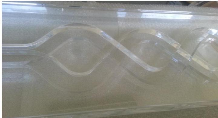
**Figure 4.40 - PIV experimental PMMA mockup**
