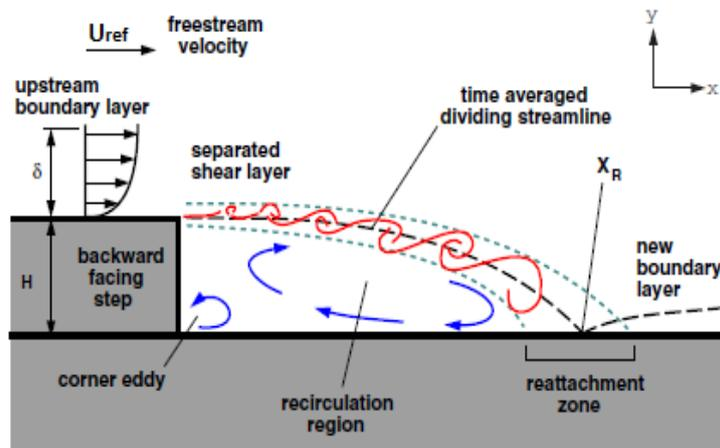
Figure 3.8 - Concept of Backward Facing Step
