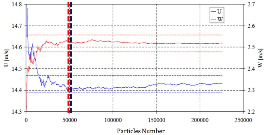
Figure 4.23 - Principal Velocity U convergence tests
