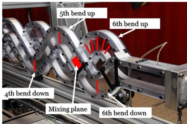
Figure 4.20 - Bend and mixing zone experimental campaign description
