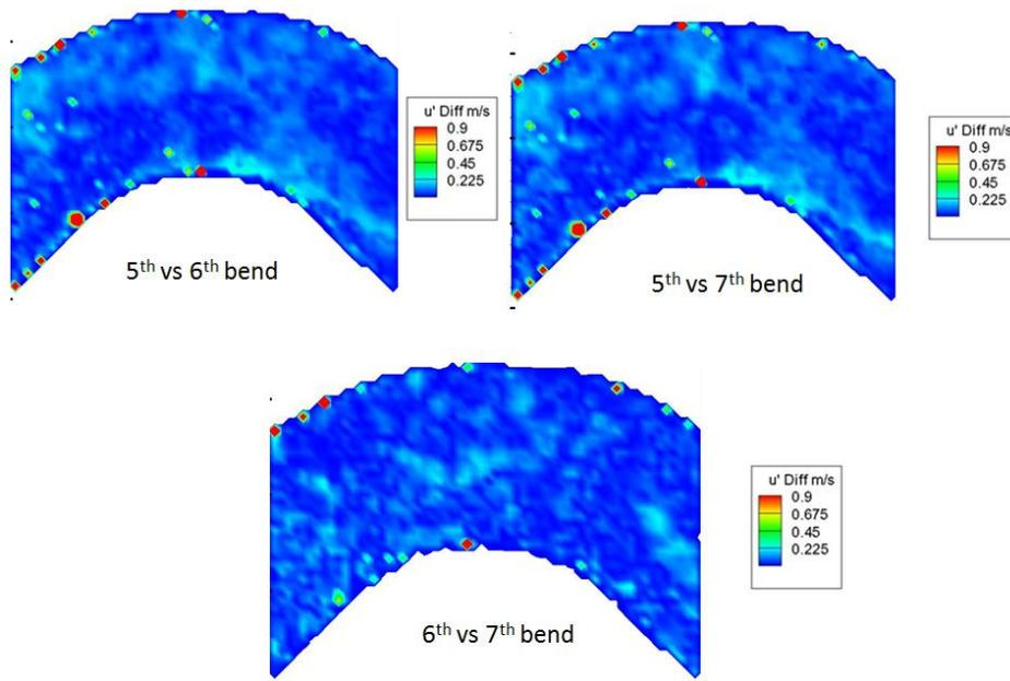
Figure 4.57 - PIV Flow development evaluation: u' velocity fluctuation
