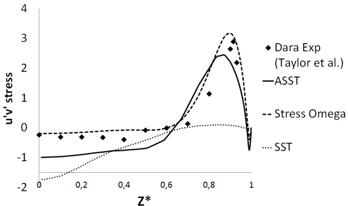
Figure 3.30 - BB line outlet mixed Reynolds stress distribution
