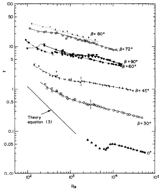
Figure 2.27 - Influence of  $\beta$  on friction factor<sup>22</sup>
