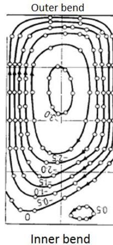
Figure 5.21 - 90° bend secondary motion according to Adachi et al.
