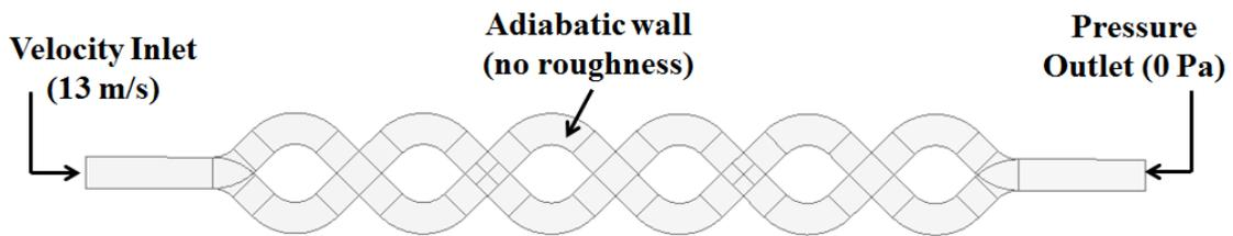
Figure 5.1 - Innovative channel computation boundary conditions
