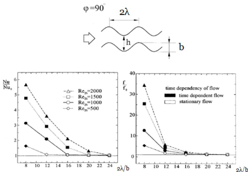
Figure 2.24- Effect of aspect ratio on thermal-hydraulic performance according to Blomerius and Mitra<sup>59</sup>
