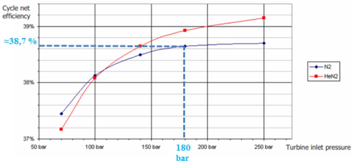
Figure 1.9 - Cycle net efficiency evaluation versus turbine inlet pressure for the gas PCS
