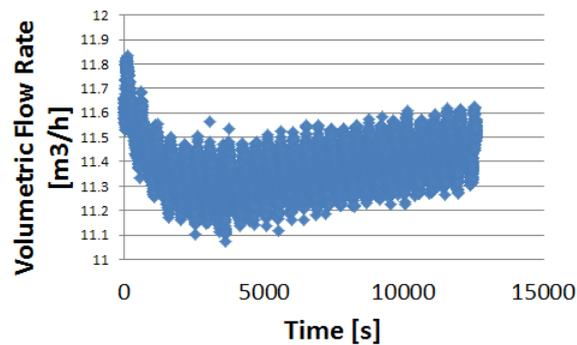
Figure 4.70 - "High heat flux case" flow stability
