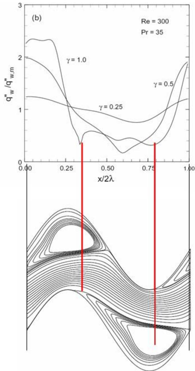
Figure 2.15 - Influence of recirculation zone on heat transfer <sup>28</sup>
