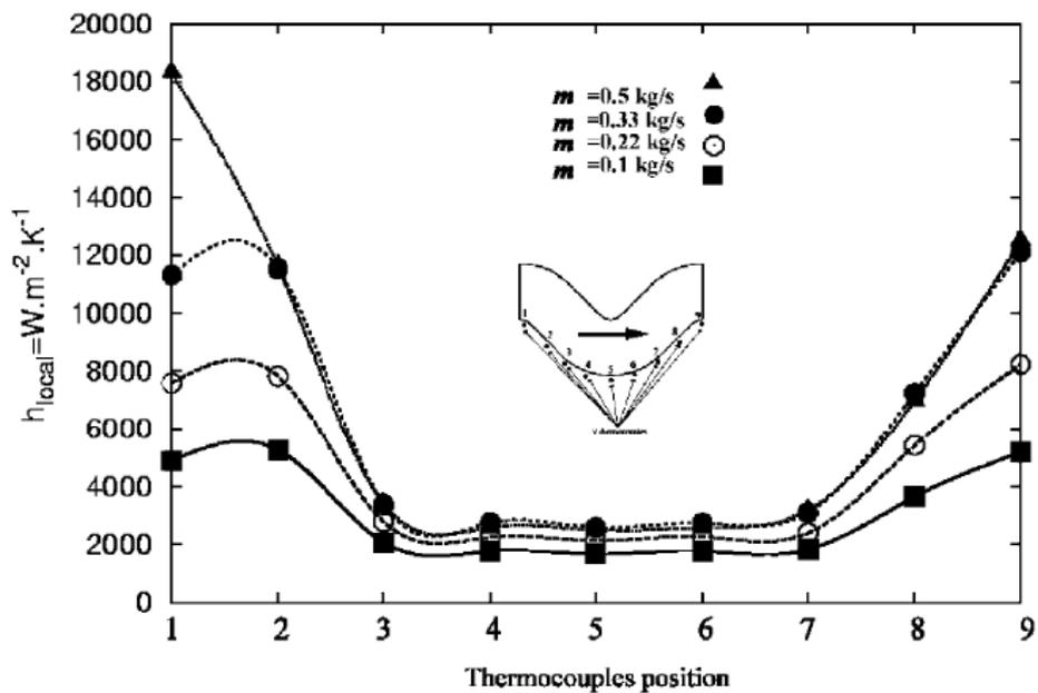
Figure 2.18 - Local heat transfer coefficient <sup>31</sup>
