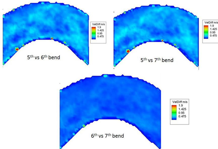
Figure 4.56 - PIV Flow development evaluation: velocity field
