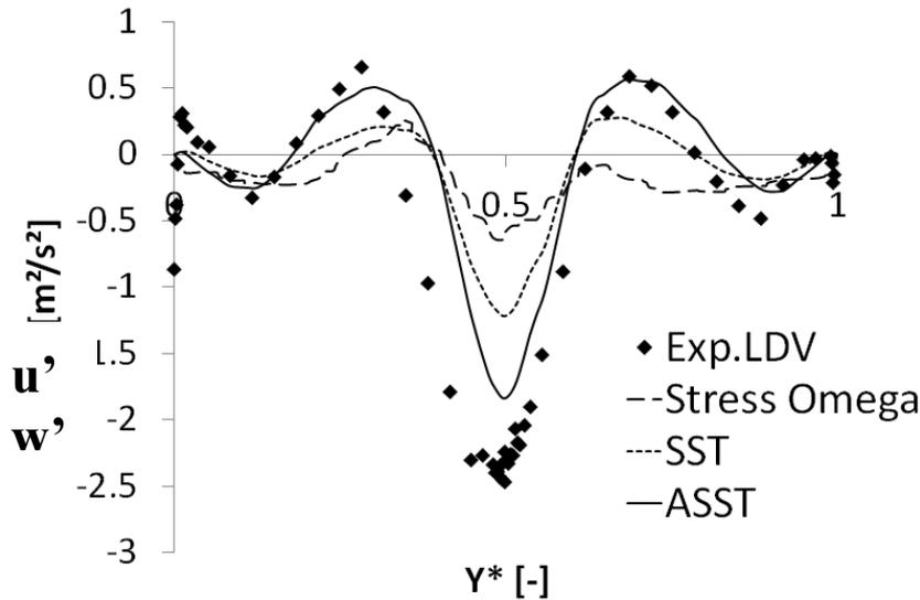
**Figure 5.7 - Experimental vs numerical mixing zone central Y profile  $u'w'$  mixed Reynolds stress**
