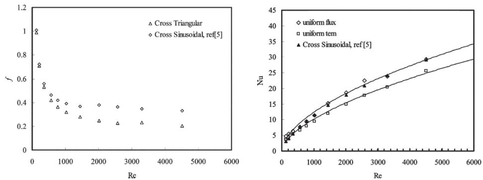
Figure 2.30 - Triangular channel performance<sup>60</sup>
