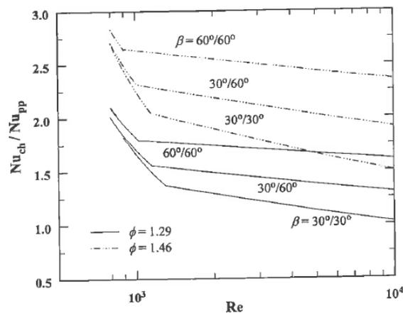
Figure 2.28 - Influence of the area enlargement factor  $\phi$  on heat transfer<sup>18</sup>
