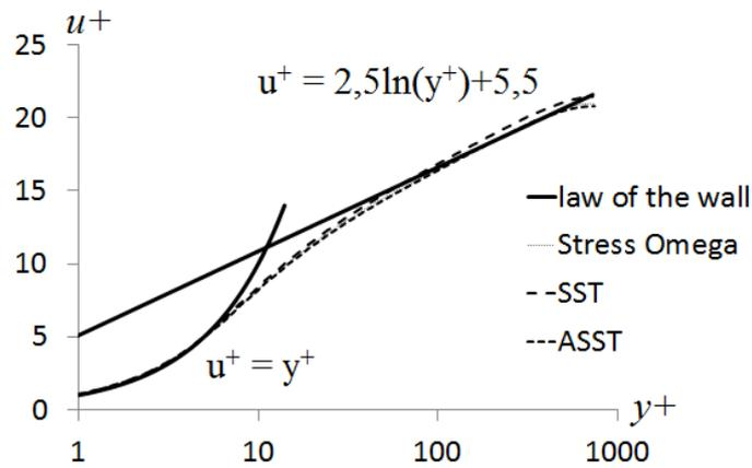
Figure 3.3 - Channel Flow law of the wall verification
