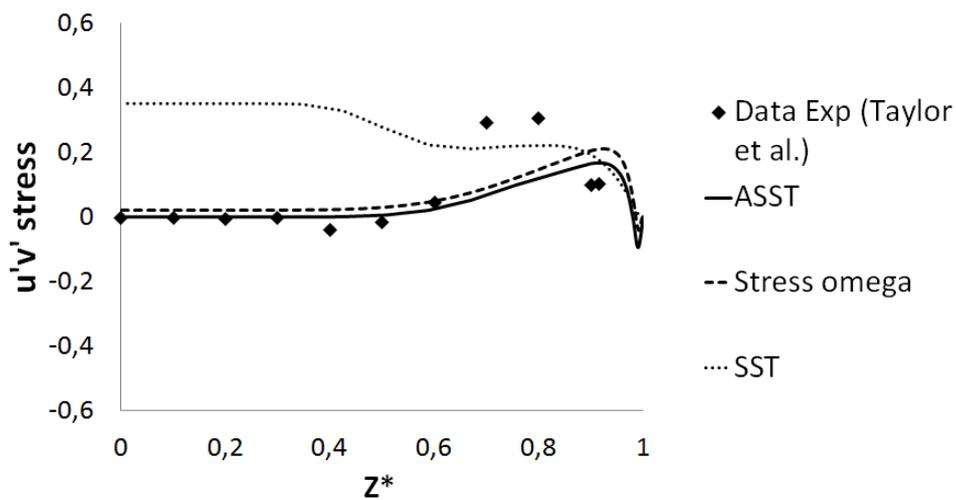
Figure 3.27 - BB line inlet Reynolds Stress distribution
