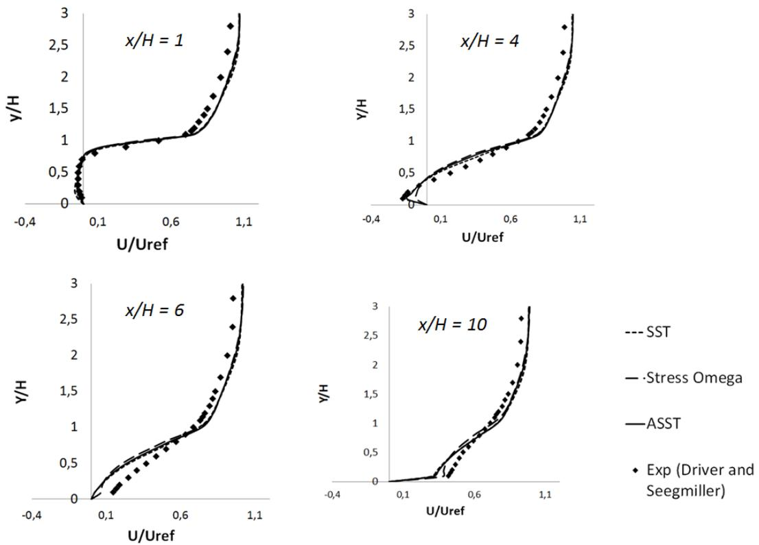
Figure 3.13 - Velocity profiles downstream the step
