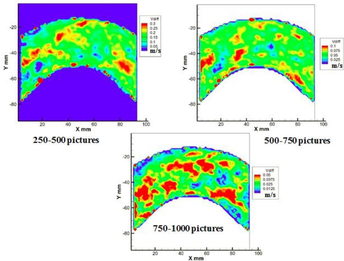
Figure 4.53 - PIV accurate measurement statistical convergence evaluation
