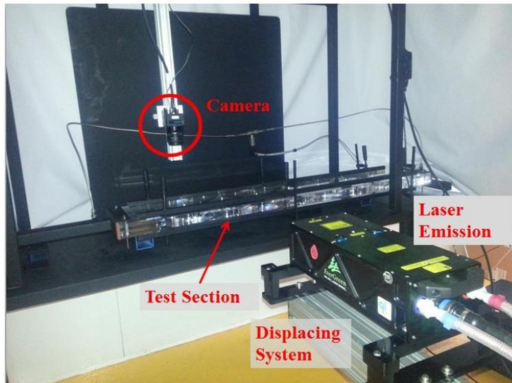
Figure 4.43 - PIV laser and camera configuration
