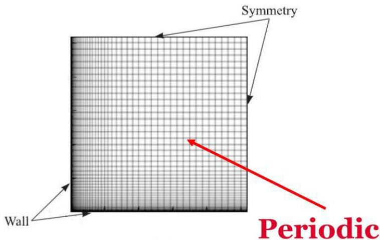
Figure 3.32 - Straight duct of squared cross-section configuration
