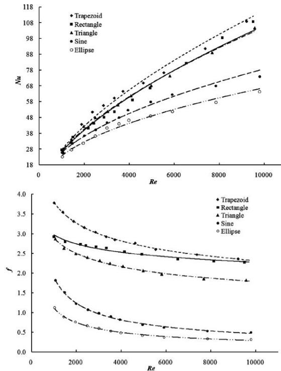
Figure 2.32 - Thermal-hydraulic performance of the different corrugation profiles<sup>61</sup>
