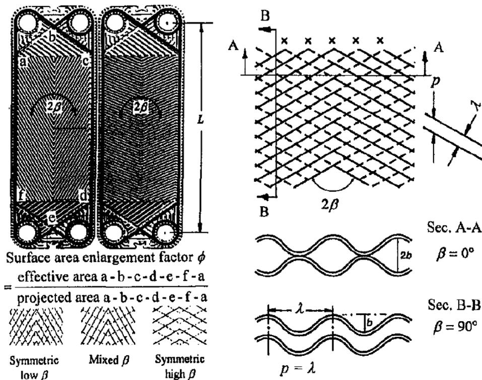
Figure 2. 7- Chevron-type plate <sup>18</sup>
