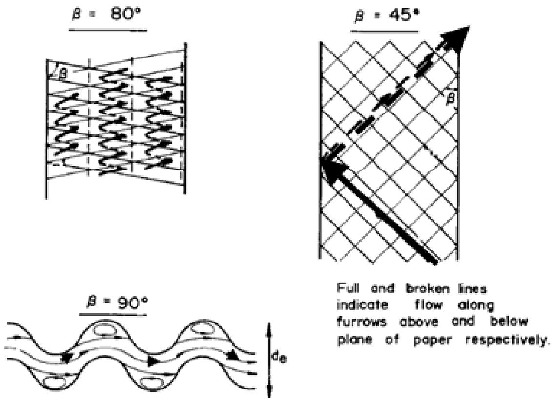
Figure 2.11 - Flow patterns depending on the chevron angle <sup>22</sup>
