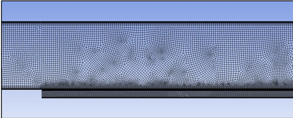
**Figure 3.9 - Backward Facing Step mesh B**
