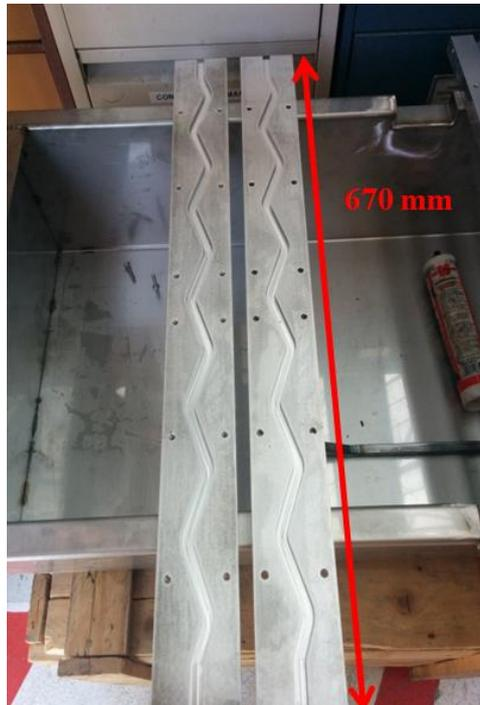
Figure 4.62 - VHEGAS innovative channel mockup
