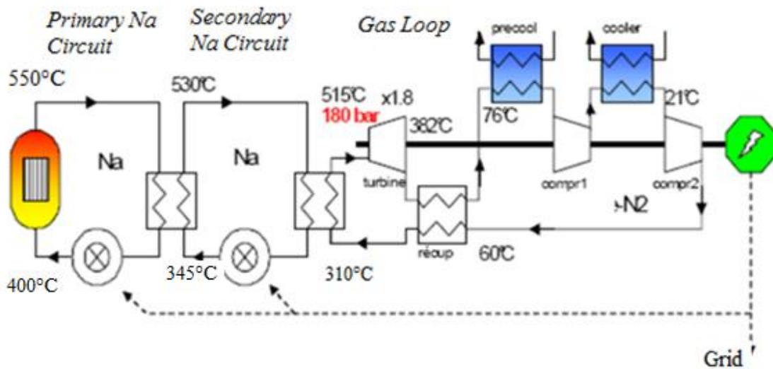
Figure 1.8 - Gas Power Conversion System (PCS) Layout
