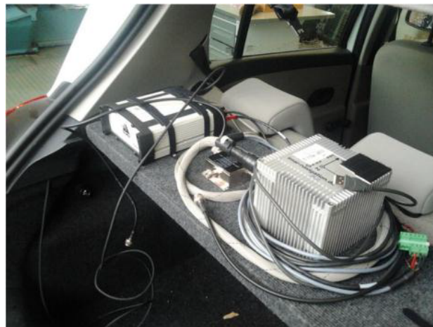
FIGURE 5.10: NovAtel SPAN as the reference system
