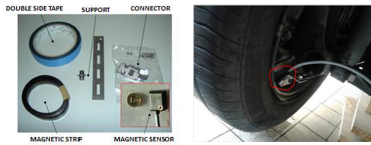
FIGURE 5.8: The iMAR iMWS-V2 magnetic strip based wheel sensor mounted on the wheel of ISAE test vehicle
