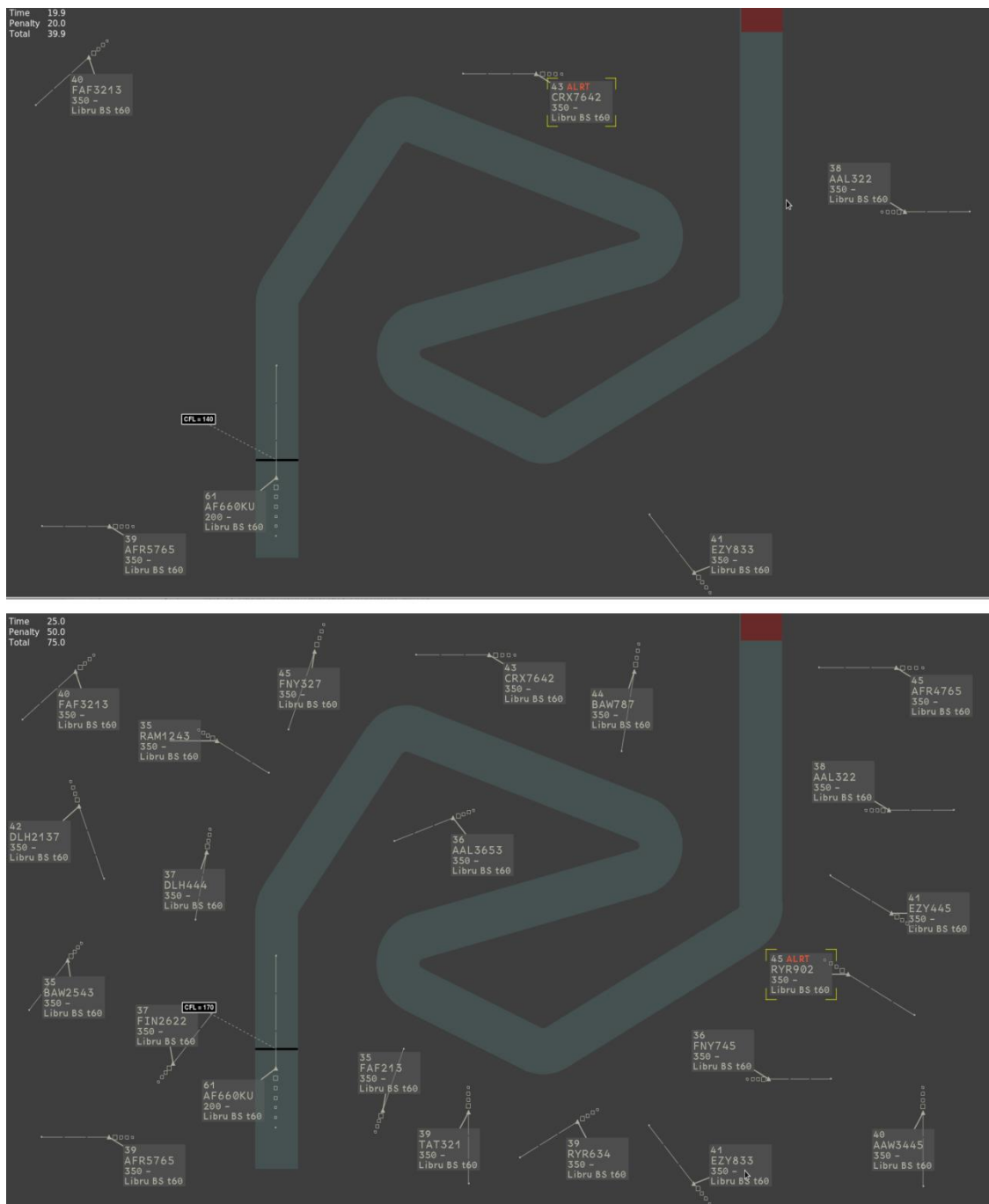
Figure 27. Screenshot of the Laby microworld simulation. On the top, an example with 5 static peripheral aircraft positioned around the corridor. Below, an example with 21 peripheral aircraft. The radar labels of the peripheral aircraft are always displayed. In both images, the main aircraft navigates through the corridor. An altitude instruction is displayed on its left (the radar label of the main aircraft appears only in this case).
