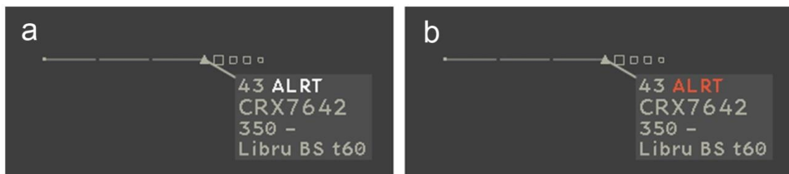
Figure 32. The visual notification inspired from the one triggered in ATC radar screens when minimum separation between aircraft is lost. The text ALRT switches from white (a) to red (b) at a rate of 200 ms white/800 ms red.
