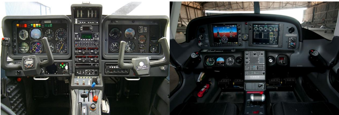
Figure 1 - Cockpit analogique (a) vs glass cockpit (b)
