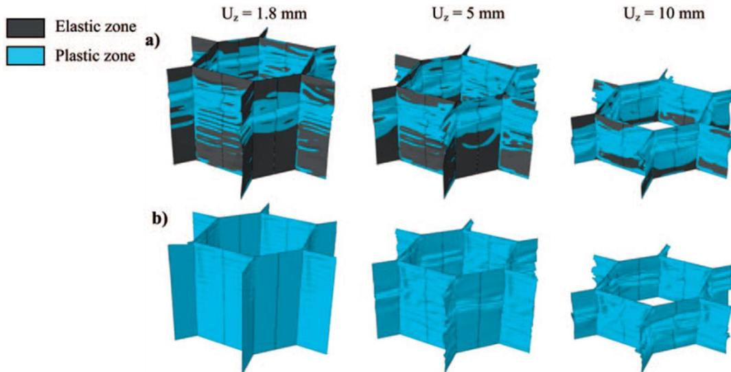
Figure I-18 : Écrasement d'un nida aluminium (a) 12 m/s and (b) 120 m/s [Kolo13]
