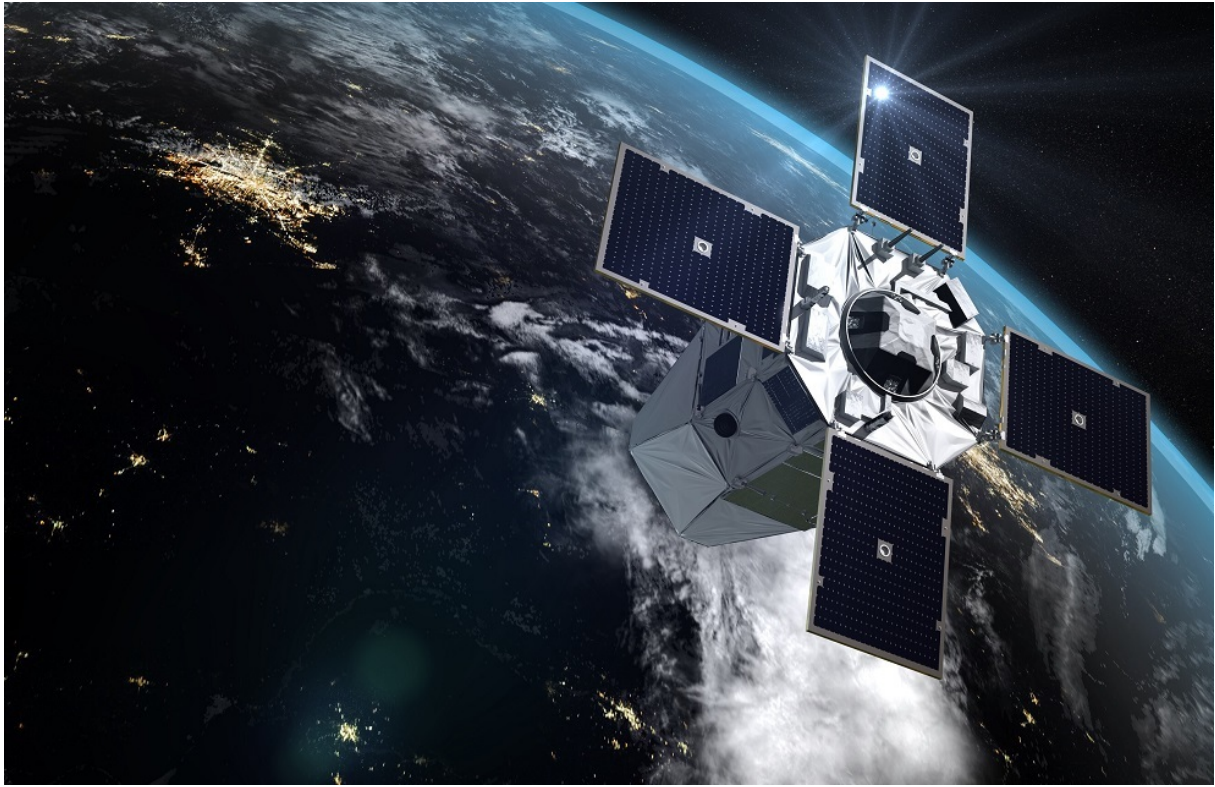
Figure 5.5: Rendering of the CSO-1 (Composante Spatiale Optique) satellite, which has a 4 fold rotation symmetry with respect to the nadir axis. Images credits: Ministère des Armées, www.defense.gouv.fr
