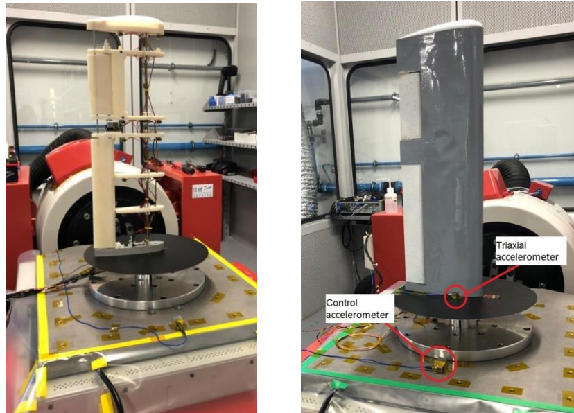
Figure 3.6 : 3D Wing setup mounted on shaker a) without skin b) with skin
