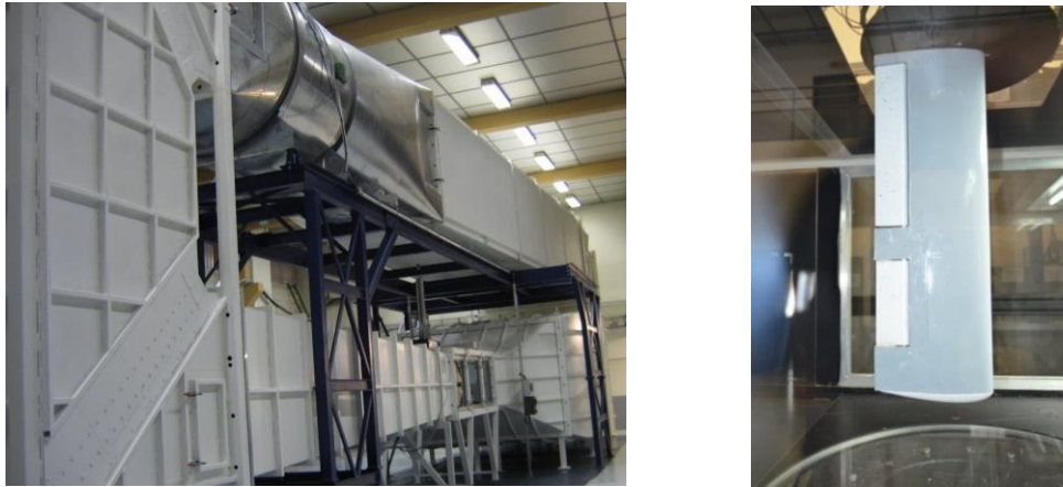
Figure 3.7 : a) Wind tunnel used for tests b) wing in wind tunnel
