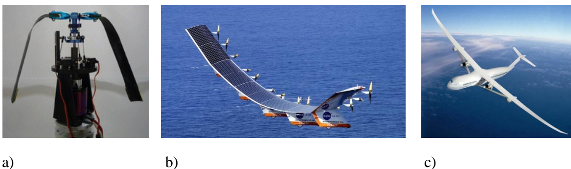
Figure 1.2 : Examples of the recent aeroelastic challenges a) highly flexible rotor blades [5] b) Helios high-altitude flying wing by NASA [6] c) high Aspect Ratio wings in Boeing Sugar Volt
