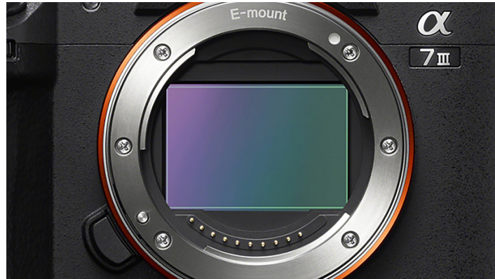
Figure 1.2: Modern full-frame 24 mm \times 36 mm CMOS Image Sensor embedded in a mirrorless camera consumer grade application.
