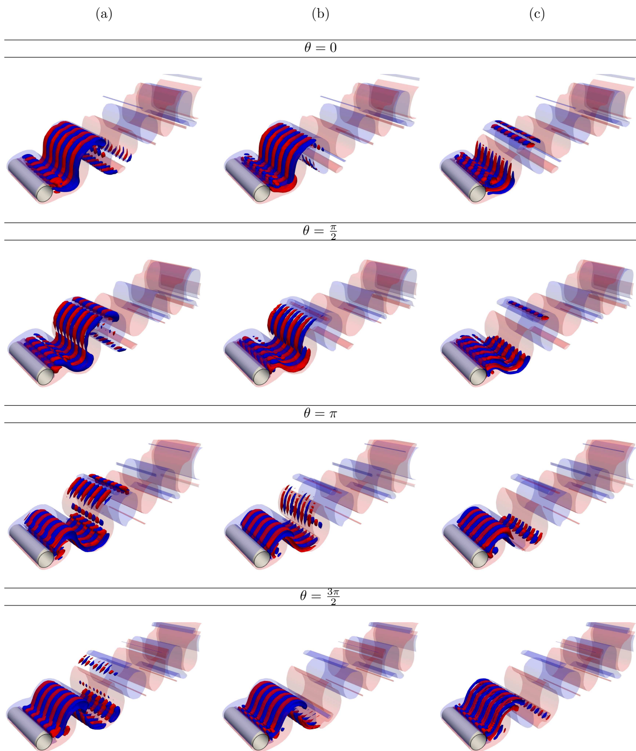
Figure 5.3 – Vorticity \tilde{\omega}/\max(|\tilde{\omega}|) of mode B with wavelength \lambda_z = 0.8D at Re = 300 and M_\infty = 0.05 for different base flow instants \theta : (a) streamwise, (b) cross-stream and (c) spanwise component. Iso-surfaces at levels \pm 0.1 (positive in red, negative in blue) superposed to translucent iso-surfaces of base flow vorticity at level \pm 0.01 .
