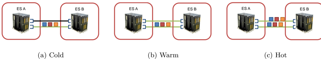
Figure 3.5: Link Redundancy Modes Example
