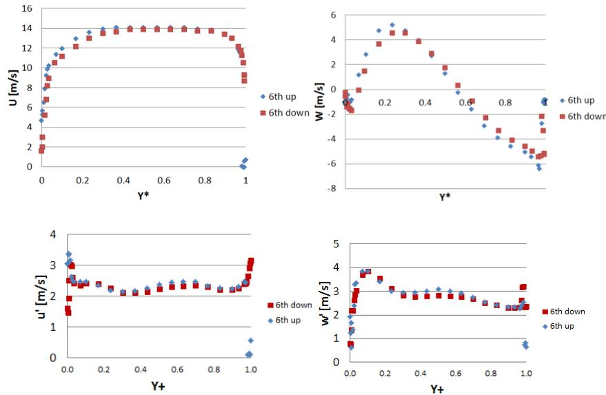
**Figure 4.36 - U and W Velocities and velocity fluctuations profiles on the z30 line with regard to flow symmetry**
