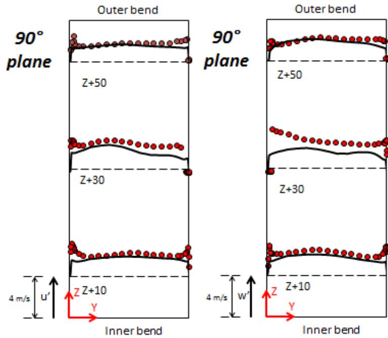
Figure E. 2 - Bend 90° plane LDV vs ASST principal (left) and radial (right) velocity fluctuation
