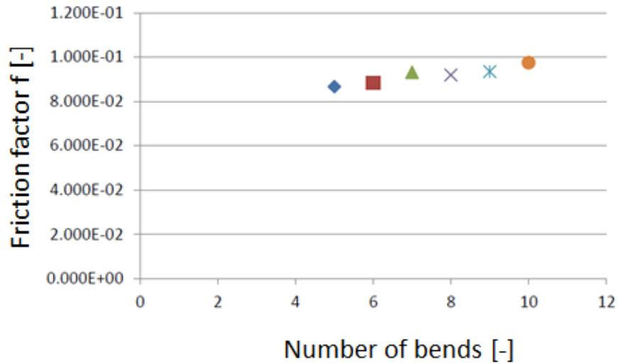
Figure 5.39 - Friction factor as a function of the number of bends for the innovative geometry
