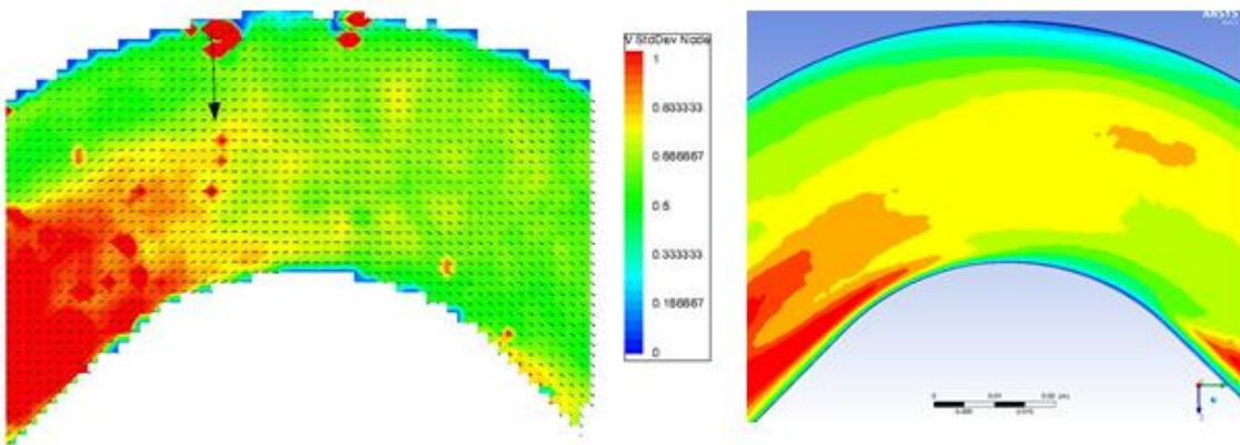
Figure E. 11 - Bend middle plane - 4 mm plane PIV vs ASST  $v'$  fluctuation
