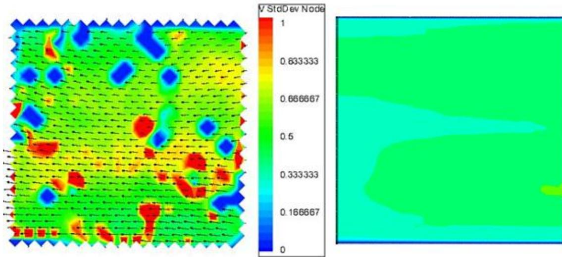
Figure E. 13 - Mixing zone top channel middle plane +8 mm plane PIV vs ASST  $v'$  fluctuation
