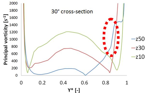
Figure 5.22 - 30° plane ASST computed principal vorticity profiles
