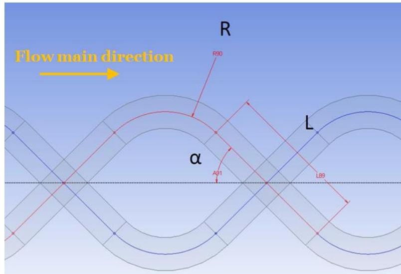
Figure 2.47 - Channel main geometrical parameters
