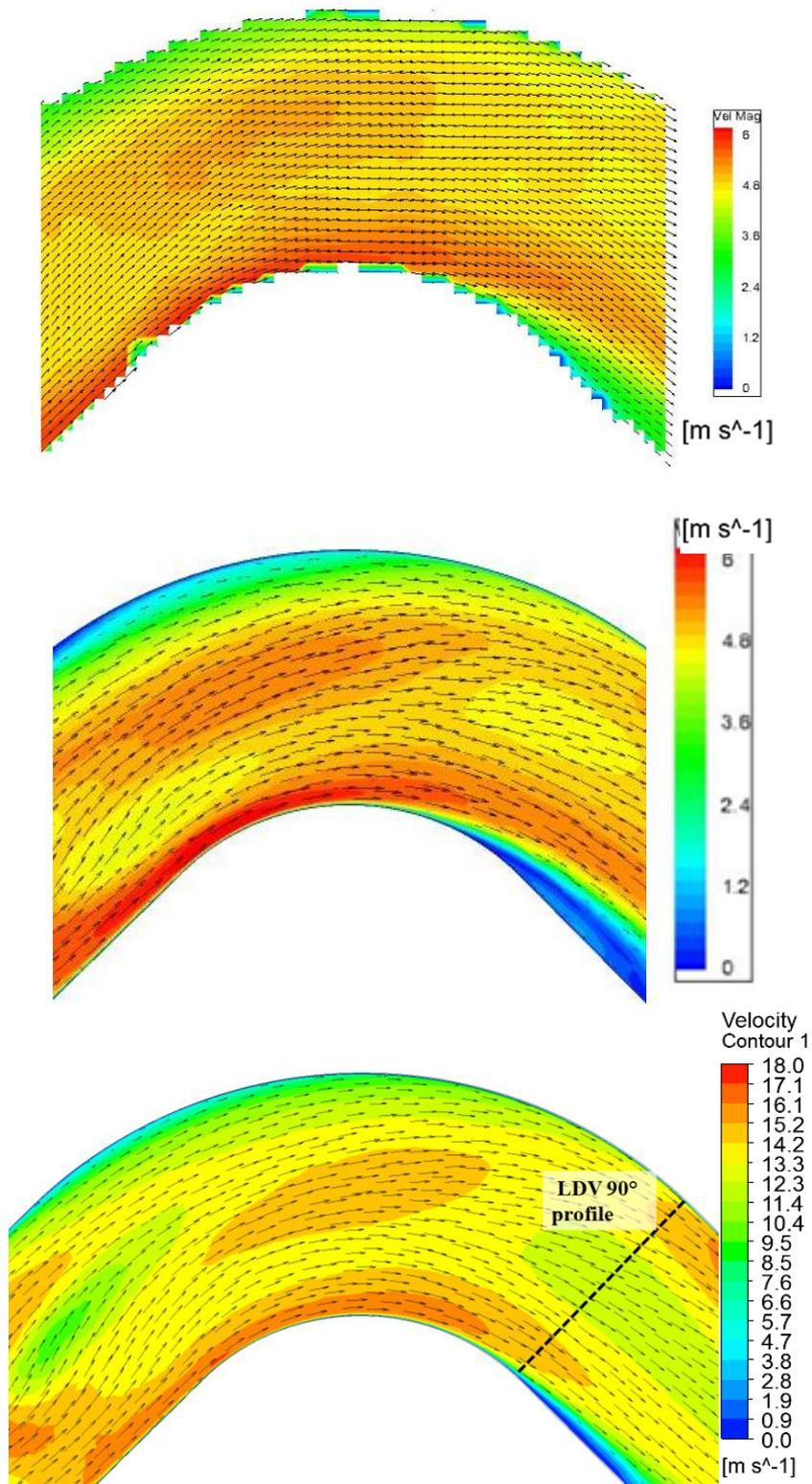
Figure 5.13 - Velocity field on bend middle plane comparison (PIV data on top, ASST computation on PIV channel geometry in the middle and ASST computation on LDV channel on the bottom at  $Y^*=15\text{mm}/30\text{mm}$ )
