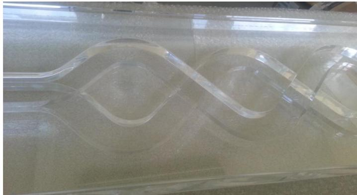
**Figure 4.40 - PIV experimental PMMA mockup**
