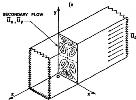
Figure 3.31 - Corner vortices as shown by Speziale<sup>89</sup>
