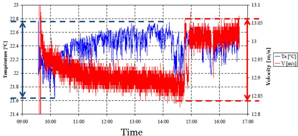
**Figure 4.17 - Flow velocity control over a day**
