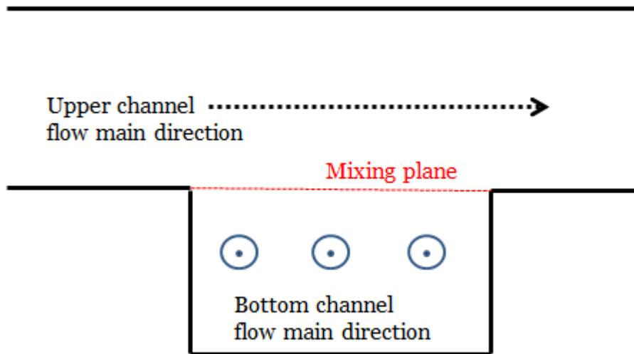
Figure 2.45 - Mixing zone and mixing plane visualization
