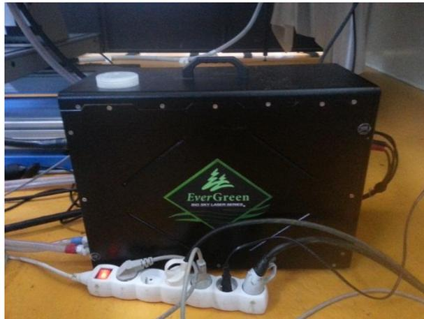
**Figure 4.42 -PIV Laser generator**
