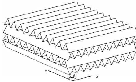
Figure 2.29 - Triangular wavy channels<sup>60</sup>
