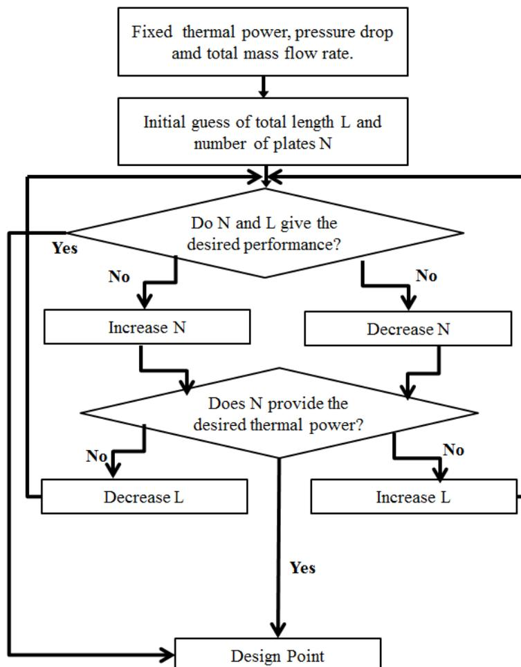
Figure 5.49 - Compact heat exchanger design process
