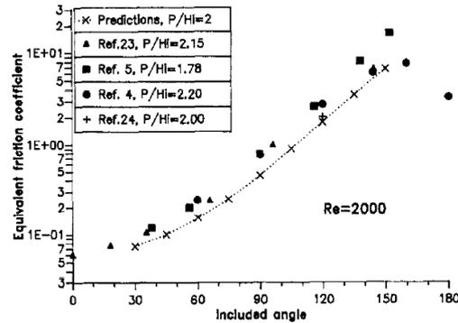
Figure 2.37 – Influence of  $\beta$  on Friction factor: CFD vs experimental results in Ciofalo et al.<sup>62</sup>
