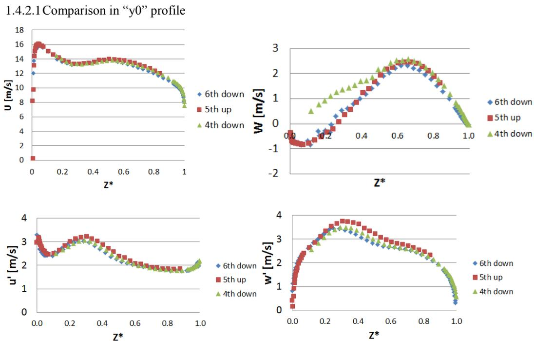
Figure 4.33 - U and W Velocities and velocity fluctuations profiles on the y0 line with regard to flow development
