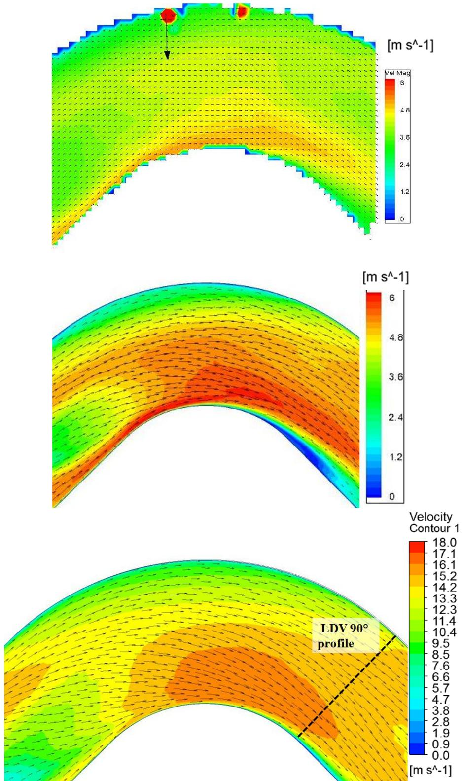
Figure 5.14 - Velocity field on bend middle plane plus 4 mm comparison (PIV data on top, ASST computation on PIV channel geometry in the middle and ASST computation on LDV channel on the bottom at 24mm/30mm)
