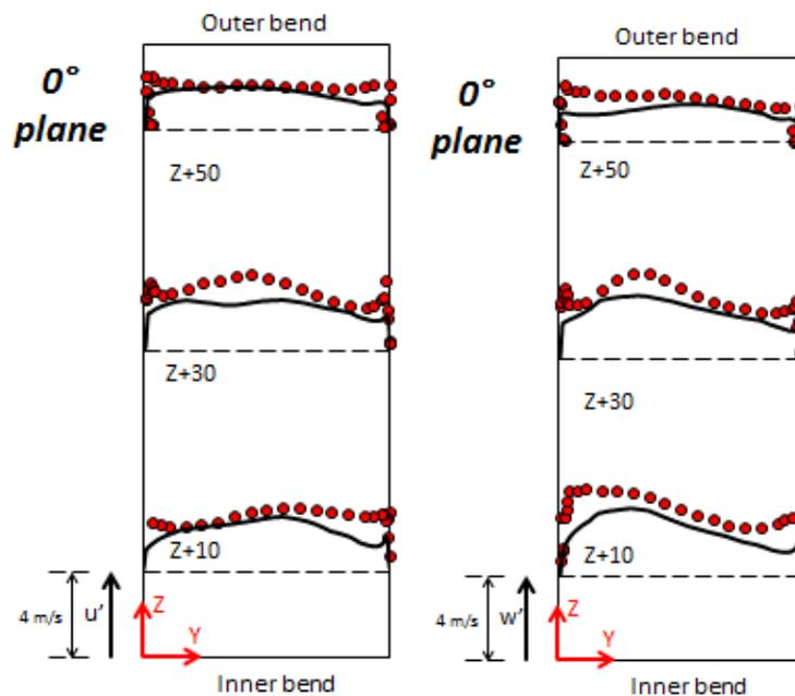
Figure E. 1 - Bend  $0^\circ$  plane LDV vs ASST principal (left) and radial (right) velocity fluctuation
