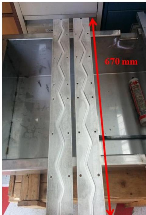
Figure 4.62 - VHEGAS innovative channel mockup
