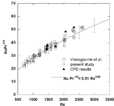
Figure 2.38 - CFD vs experimental results in Kanaris et al.<sup>49</sup>
