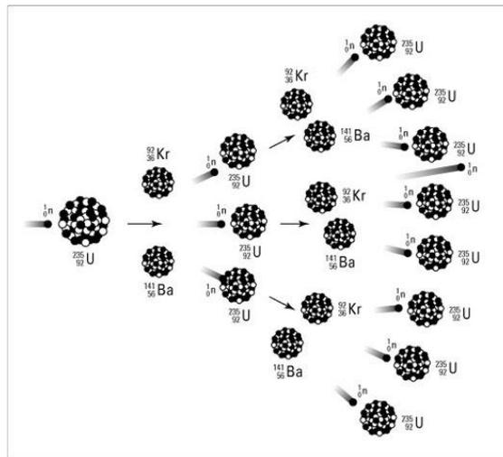
Figure 1.2 - Example of a fission chain<sup>1</sup>
