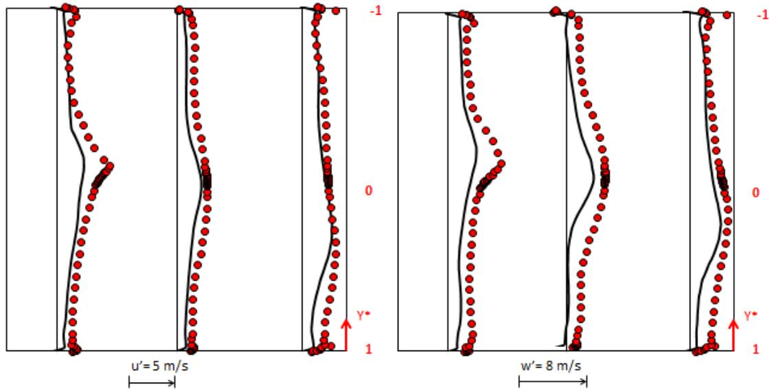
**Figure E. 4 - Mixing zone middle plane LDV vs ASST principal (left) and radial (right) velocity fluctuation**
