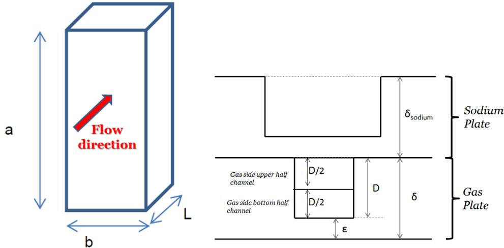
Figure 5.50 - Compact heat exchanger major dimensions
