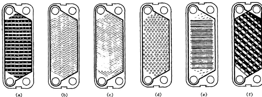
Figure 2.2 - Different types of plate: (a) Washboard, (b) Zig-zag, (c) Chevron/Herringbone, (d) Protrusions and depressions, (e) Washboard with secondary corrugations, (f) Oblique washboard<sup>13</sup>
