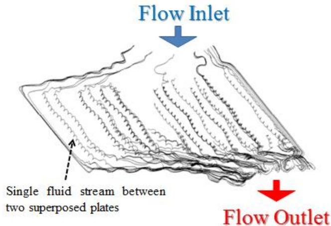
Figure 2.13 - Flow pattern from CFD simulation for  $\beta=60^\circ$  and  $Re=1565$ <sup>19</sup>
