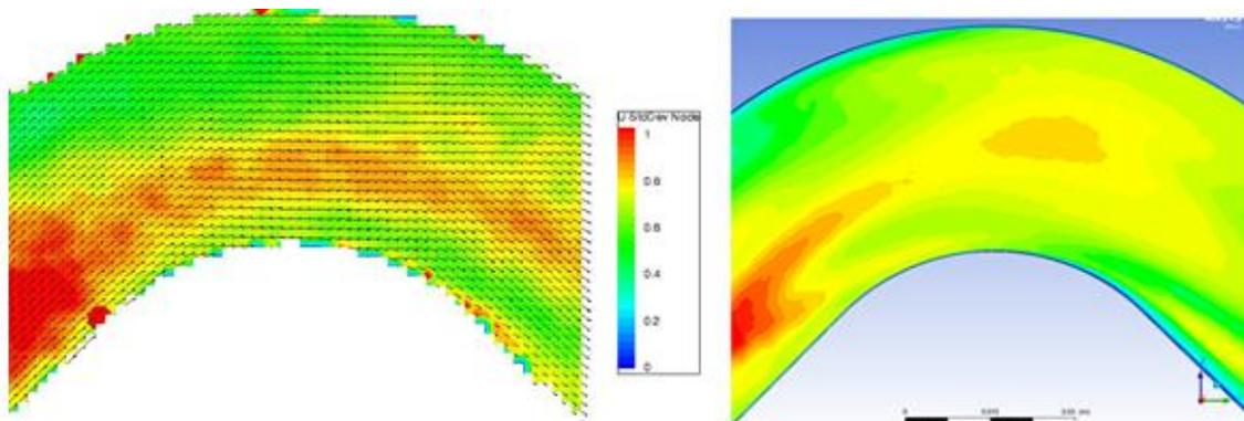
Figure E. 8 - Bend middle plane PIV vs ASST  $u'$  fluctuation
