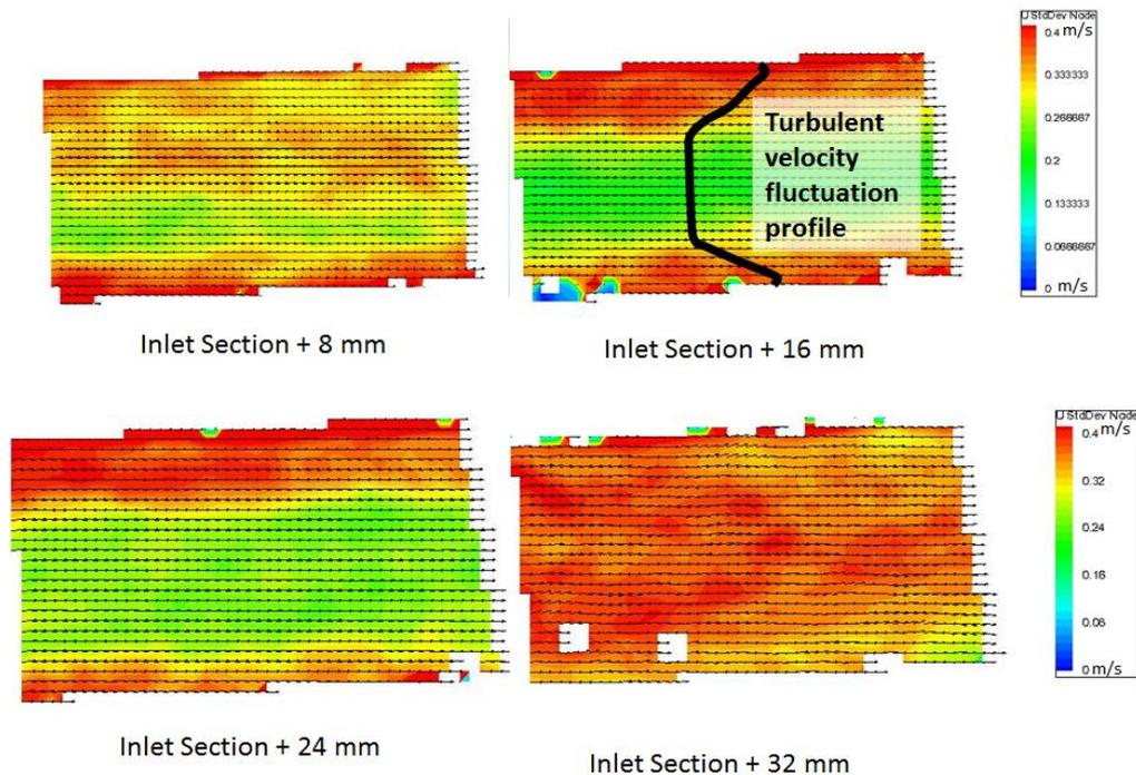
**Figure 4.55 - Inlet Flow  $u'$  velocity fluctuation field distribution**
