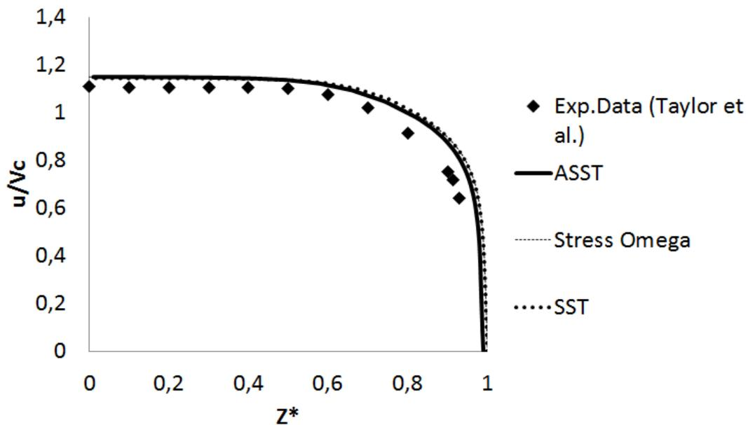
Figure 3.25 - BB line inlet section principal velocity distribution
