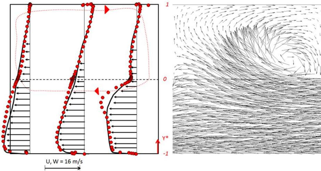
Figure 5.27 - LDV/ASST data on principal and radial velocity at mixing zone outlet plane (on the left) and ASST computed secondary velocity vectors (on the right)
