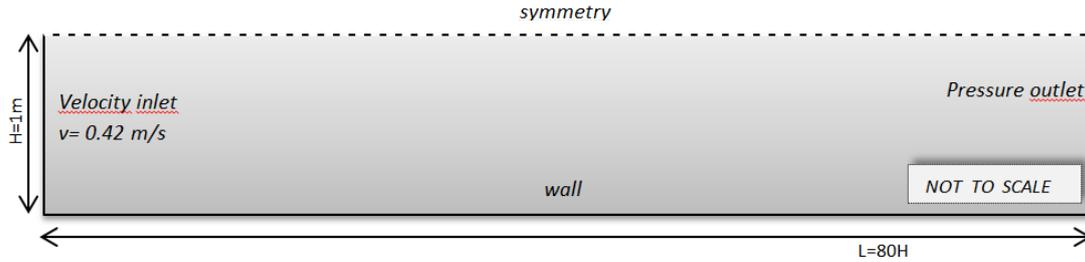
**Figure 3.1- Channel Flow Geometry**
