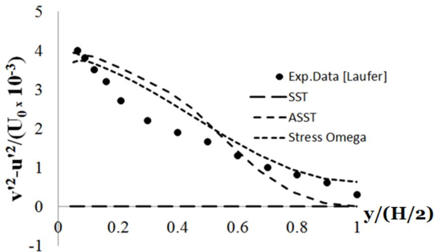
Figure 3.7 - Channel Flow anisotropy distribution at Re = 14 000 (Laufer<sup>84</sup>)
