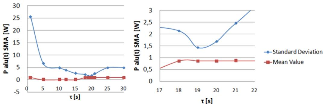
Figure 4.72–“High Heat Flux” case evaluation of thermal transient by mockup thermal power absorption
