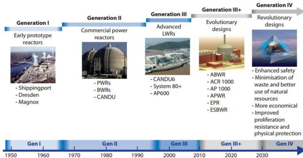
Figure 1.6 - Generations of nuclear reactors<sup>4</sup>
